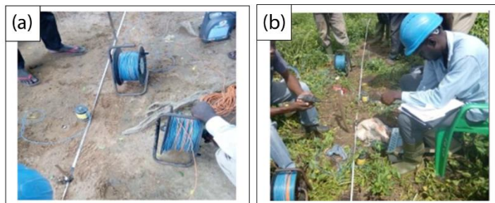
Figure 4 : Implementation of the Schlumberger configuration. (a) device installation, (b) data recording
