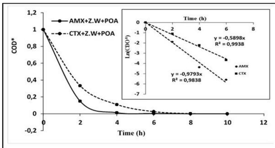
**Figure 2 :** Evolution of the normalized COD versus time during the photochemical process. In insert the evolution of the graph  $\text{Ln}(\text{COD}^*) = f(t)$  for the two types of solutions.
