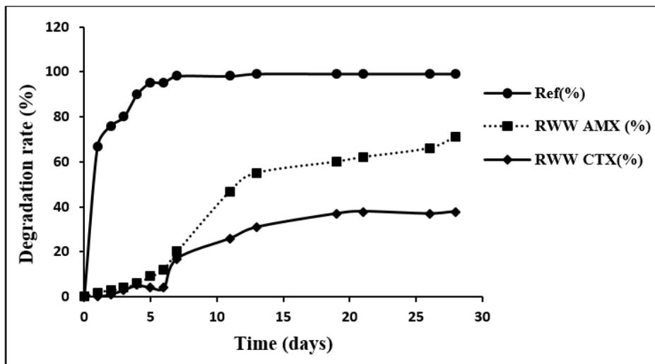
**Figure 1 :** AMX and CTX wastewater degradation rates versus time
