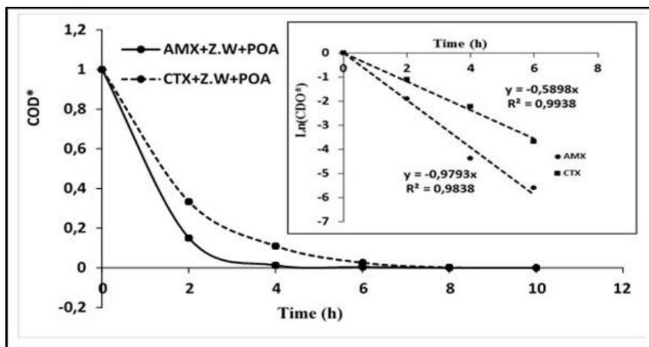
**Figure 2 :** Evolution of the normalized COD versus time during the photochemical process. In insert the evolution of the graph  $\text{Ln}(\text{COD}^*) = f(t)$  for the two types of solutions.
