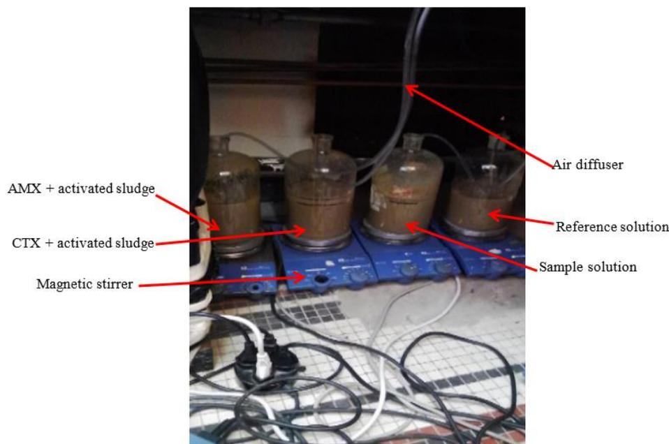
**Picture 1 :** Biological treatment device by the method of Zahn Wellens
