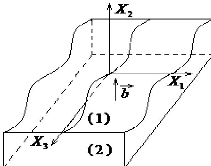
**Figure 1 :** Two elastic media (1) and (2) welded along a non-planar sinusoidal surface and containing an interface sinusoidal dislocation at the
