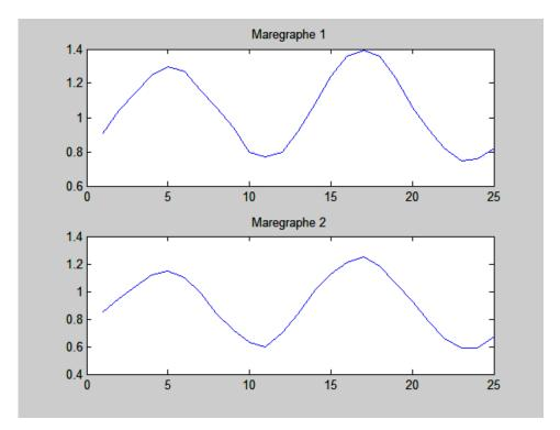
**Figure 3** : water level line of the 2 tide gauges from August 28th to 29th at 4pm. (X-coordinate: length - hour; Y-coordinate: level- m)
