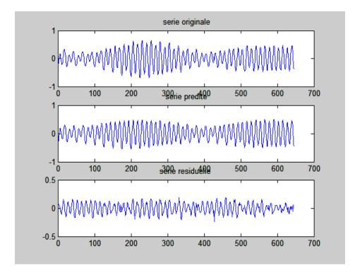
**Figure 4** : *Time oscillations of the water level (high), prediction of the corresponding tide (center) and residual oscillations (low) of tide gauge 1(X-coordinate: frequency – hour; Y-coordinate: level- m)*
