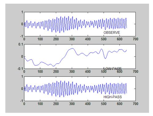
Figure 2 : Time oscillations (OBSERVES), low frequency (LOW-PASS) and high frequency (HIGH-PASS) of the water level recorded by tide gauge 1. (X-coordinate: frequency – hour; Y-coordinate: level- m)
